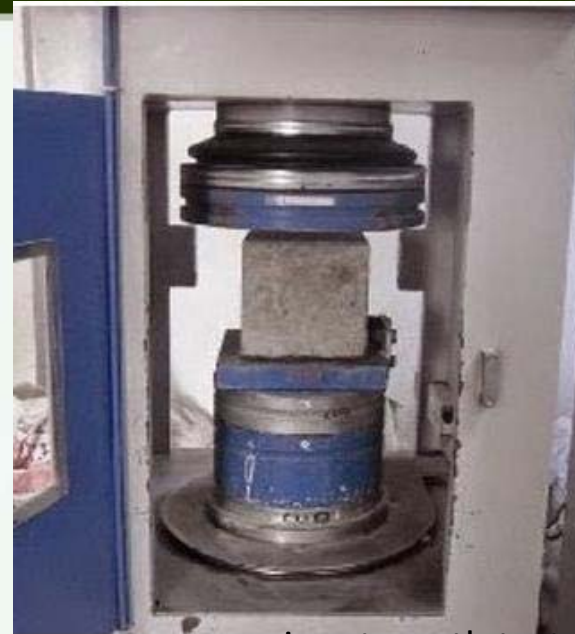
compressive strength test for cube
