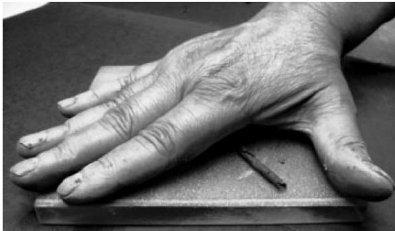
Figure (4.4) Rolling of soil mass on ground glass plate to determine plastic limit
