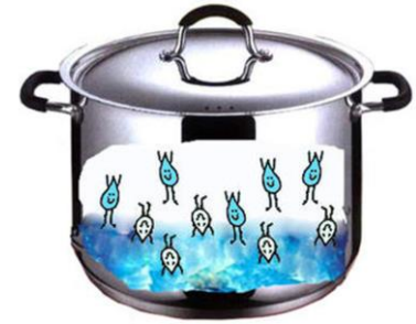
Fig. 2. Vapor pressure is constant when there is an equilibrium of water molecules, in a closed container.
